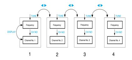
You can directly switch between the channels presets (
